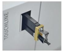
Up to four perforating or slitting heads are available; all of them plug and play. The setup will be done within just a few seconds on the touchscreen control panel.
